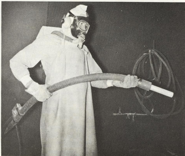
This sandblasting job requires Domingo J. Werleman of Mechanical-Shops to wear this Fresh Air Hose Mask in addition to other protective clothing.
