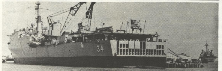
The USS PONCE (top), and the USS HERMITAGE (below), visited Aruba from Oct. 1-3. The USS Ponce is an Amphibious Transport Dock with a helicopter landing deck and hangar to house them. Underneath the landing deck is a floodable well for launching, receiving and transporting amphibious vehicles. The ship was built in 1971 and is on her first operational deployment to the Caribbean. Aki riba ta USS PONCE, cu USS HERMITAGE (mas abao), cu a bishita Aruba Oct. 1-3.
